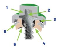
Dekfast\* Multi-Seal™ Washer: Four sealing points to assure positive seal even when driven at extreme angles. Protects and seals (3) Under the head, (4) Against the shank, (5) Against the roof sheet. (6) Engineered to distribute the load. Ideal for 5V roof applications
